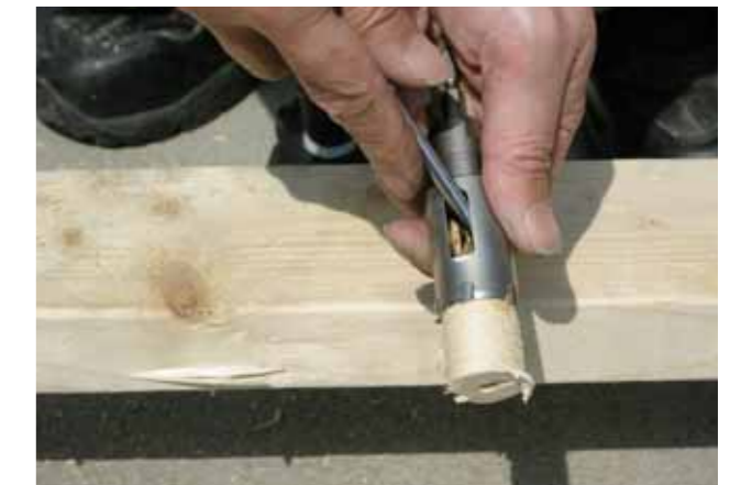
Easy slug removal with side slot.
