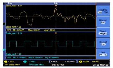
To find intermittent faults the TrendPlot  $^{\text{\tiny{TM}}}$  function can monitor measurements for long periods of time.
