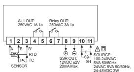
X1: AC power: 100-240VAC 5VA 50/60Hz AC/DC power: 24VAC 5VA 50/60Hz, 24-48VDC 3W
